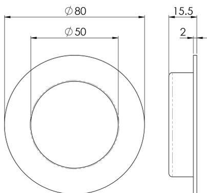
78mm Dia. circular shaped low profile flush pull which is used mainly on sliding doors. The main cup is recessed back into the door to leave a flush appearance. For use on doors, wardrobes or cupboards.
