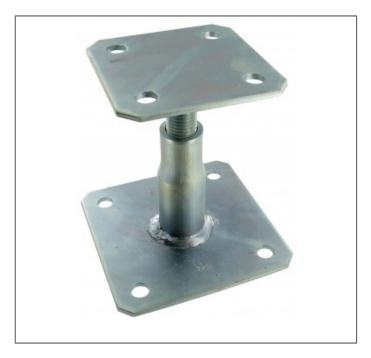
The APB features a post mounting plate on a screw allowing it to be adjusted to a specific standoff height ranging from 100-150mm. Suitable for post sizes 100 x 100mm to 200 x 200mm.
