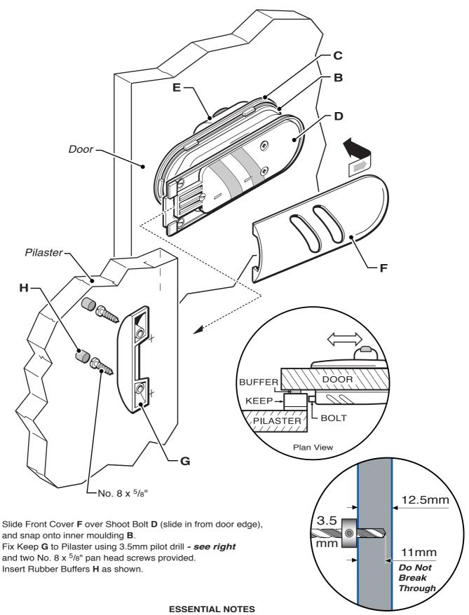
Do not over tighten Handle E fixing screws.
