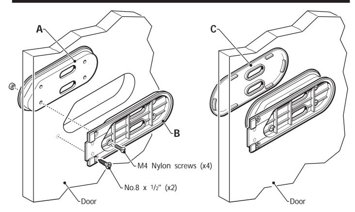
Fix white inner mouldings **A** & **B** either side of hole in door as shown. Fix with M4 nylon screws and nuts provided. Fix inner moulding **B** to door with No. 8 x ½" csk screws provided. For **13mm** board use 3.5mm pilot drill.
