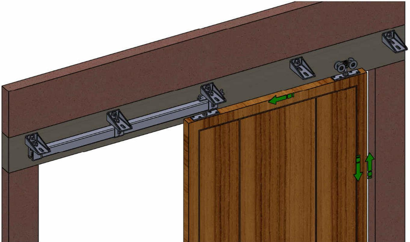
Insert the first track through the brackets making sure it fits into the closed end piece. You might have to disassemble some of the brackets for easy access as shown in fig.14.
