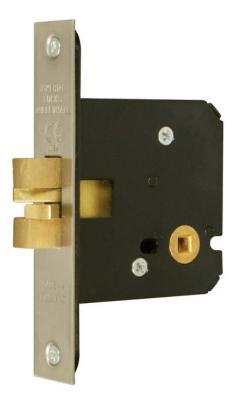
**Description** Bathroom mortice sliding door lock for use on wooden sliding doors. CE Marked door lock Fire rated to BS EN 1634-1:2000 & Performance rated to BS EN 12209. Bolt operated by turn from either side. Supplied with striker plate and fixing screws. Finishes stainless steel (SS) or satin brass (SB). Other finishes available.
