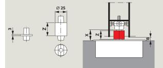
Calculating the necessary length of spindle extension: Extension = **X** – Floor clearance (normally 8 mm) Collar height **Z** of the extended spindle inserts = Spindle extension length + 3 mm (collar height of the standard spindle insert)
