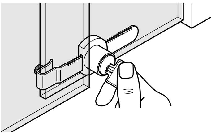
On closing the doors, slide the cylinder to the left and lock onto the rack
