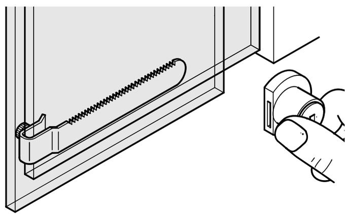
To open, remove the cylinder from the right hand end of the rack
