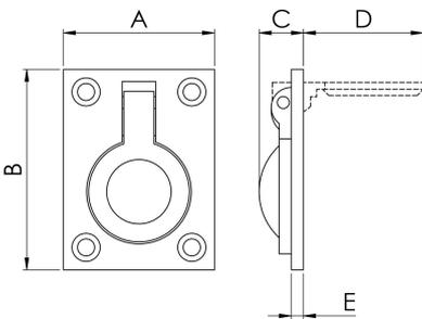
Flush ring pull handle is used for pulling flush panels, sliding doors, trap doors, cabinet doors, traditional kitchen drawers and any situation where a handle with a projection would not be suitable. Basic and easy to operate, simply pull on the ring which will elevate and in turn pull the item to which the mounting plate is affixed. Larger version available for heavier applications. Comes with a 10 year mechanical guarantee.
